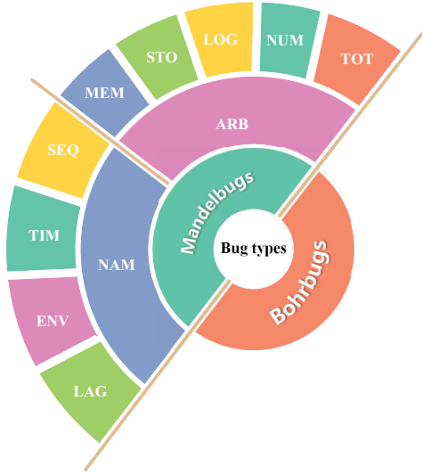
Fig. 2. Based on the complexity of fault triggering conditions, bugs are classified as Bohrbugs and Mandelbugs. Mandelbugs can be further categorized as non-aging-related Mandelbugs (NAMs) and aging-related bugs (ARBs). There are also subtypes in NAMs and ARBs.
